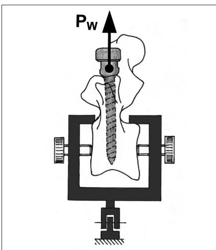
**Fig. 3.** Schema of loading system.
