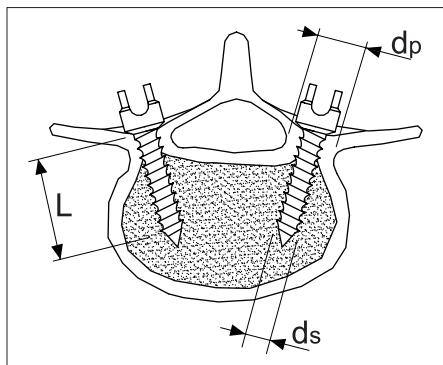
**Fig. 2.** Schema of inserting screw in vertebra and geometrical parameters.
