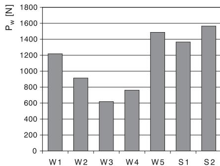
**Fig. 4.** Average value of pull-out force for investigated screws
