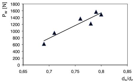
Fig. 6. The changes in pull-out strength value in relation to  $d_s/d_p$  ratio
