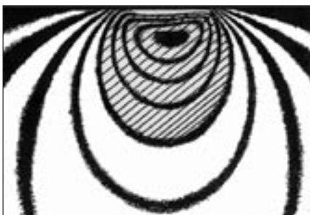
Fig. 2. The isochromats lines of constant shear stresses in subchondral bone. The cross-hatch area predefine the volume of tissue degradation and creation of granulations.
